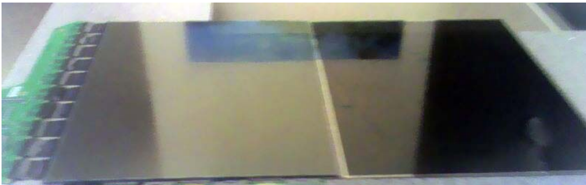
Figure 14. The two glass plates separated before replacing the liquid crystals between them .
